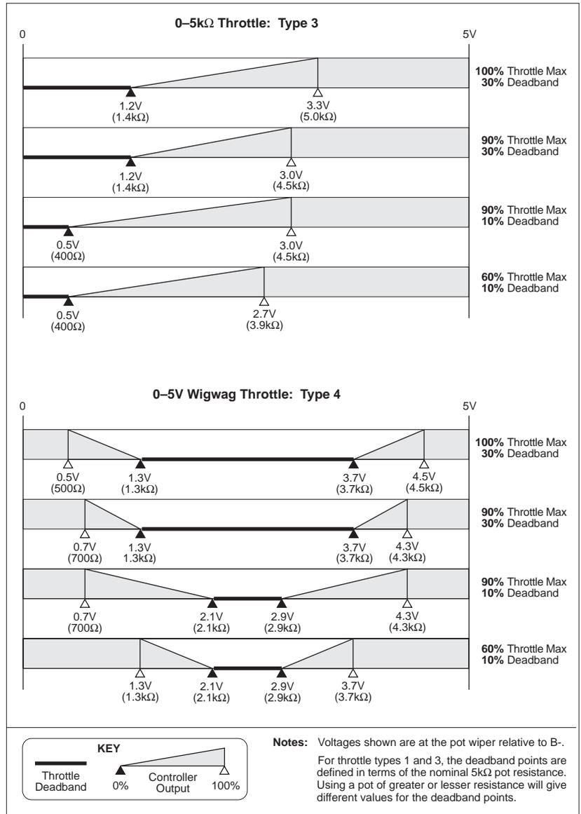
The programmer displays the throttle max parameter as a percentage of the active throttle voltage range. The throttle max parameter can be adjusted from 100% to 60%, in 2% increments. The nominal throttle wiper voltage range depends on the throttle type selected. See Table 1 (page 10) for the characteristics of your selected throttle type.
