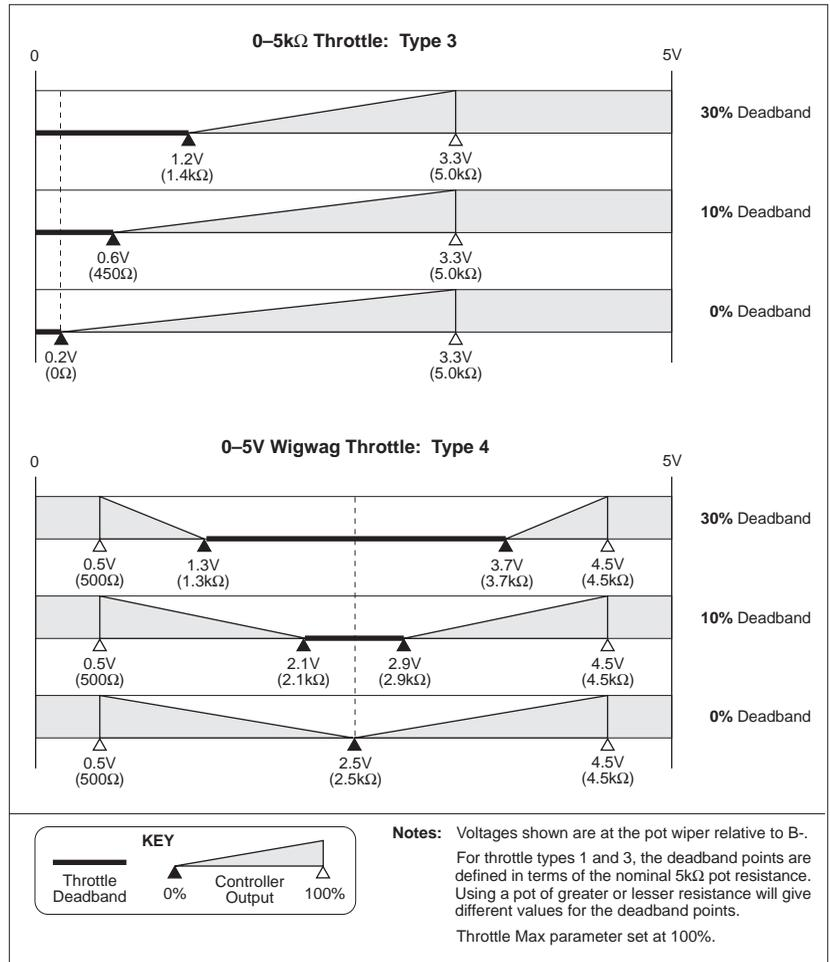
The programmer displays the throttle deadband parameter as a percentage of the nominal throttle wiper voltage range and is adjustable from 0% to 30%, in 2% increments. The default deadband setting is 10%. The nominal throttle wiper voltage range depends on the throttle type selected. See Table 1 (page 10) for the characteristics of your selected throttle type.
