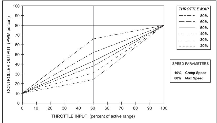
The Throttle Map operates within the window established by the Creep Speed, Max Speed, Throttle Deadband, and Throttle Max parameters, as shown in Figure 18. Creep Speed and Max Speed define the controller’s output range, while Throttle Deadband and Throttle Max define the throttle’s active range. These four parameters, together with the Throttle Map, determine the controller’s output response to throttle demand.
