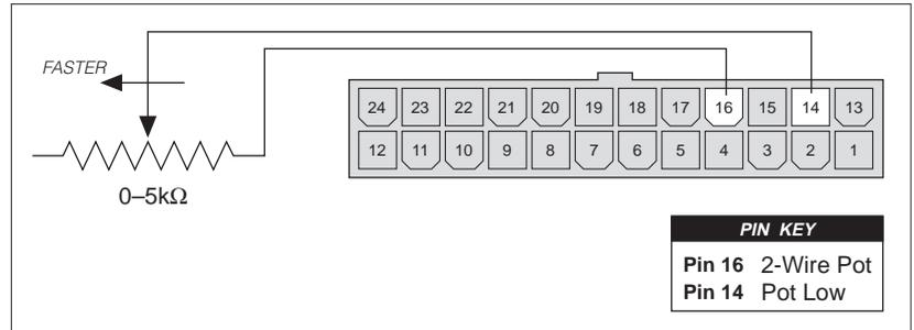
If the total resistance between Pins 14 and 16 is greater than 7.5 k $\Omega$ , the controller’s 4.4 V upper fault limit will be exceeded and the controller output will be disabled. This provides broken wire protection, and also serves as an indication that the potentiometer’s nominal value has increased and the pot needs to be replaced.
