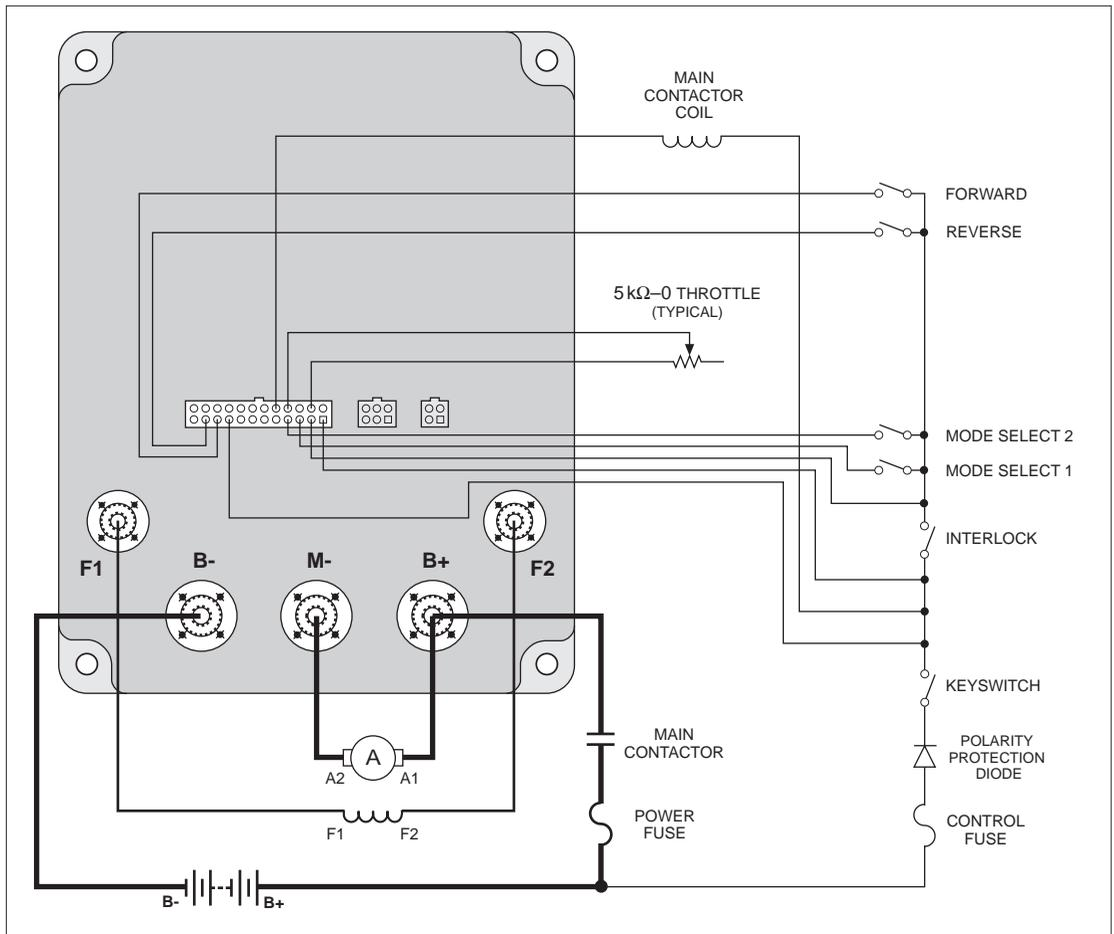
Fig. 3 Standard wiring configuration, Curtis PMC 1244 controller.
