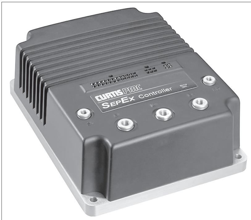
The 1244 MultiMode™ controller offers smooth, silent, cost effective control of motor speed and torque. A four quadrant, full-bridge field winding control stage is combined with a two quadrant, half-bridge armature power stage to provide solid state motor reversing and regenerative braking power without additional relays or contactors. The 1244 controller can also be specified to be compatible with CAN Bus communication systems.
