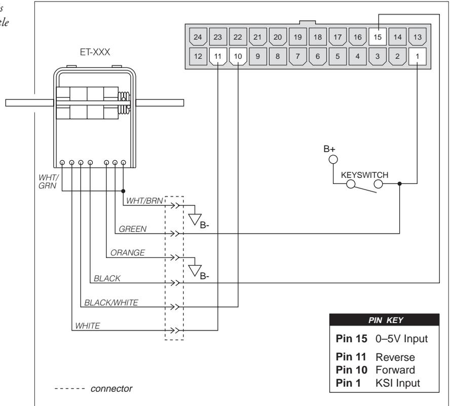
The ET-XXX can be integrated into a control head to provide wigwag-style throttle control. Alternatively, a complete control head assembly is available from Curtis. This control head assembly—the CH series—combines the ET-XXX throttle with a variety of standard control head switch functions for use in walkie and lift truck applications.
